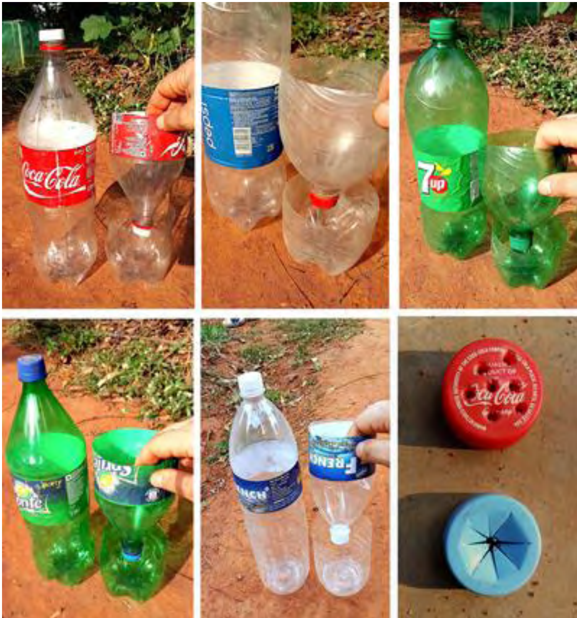
Photo 4 - Different types of bottle used (from top to bottom and from left to right): Coca Cola lt. 2.25, Pepsi lt. 2.25, 7 UP lt. 2.25, Sprite lt. 2.25, French lt. 2. At the bottom right corner: Caps pierced with a nail (top) and in the shape of a star through a trench (bottom).
