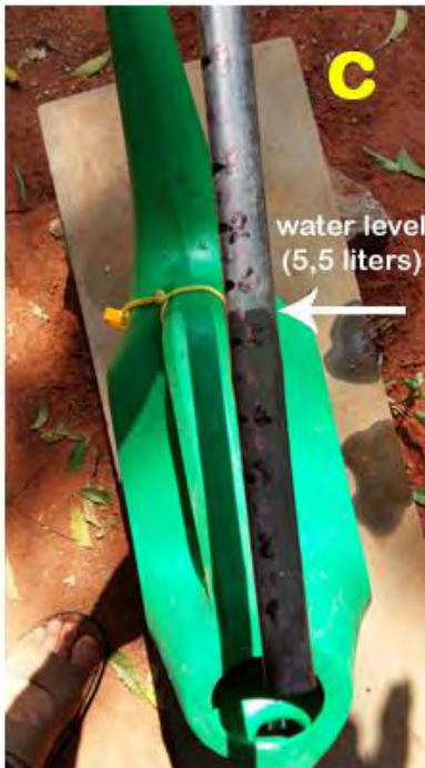
Photo 27 – a) 10-liter watering can. b-c) Graduated bar for measuring irrigation volumes (liters).
